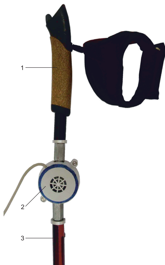
Figure 2 Detailed view of strain gauge force transducer mounted below the grip of NW pole. 1 – grip, 2 – strain gauge force transducer, 3 – lower part of the pole (seven different lengths were available)
