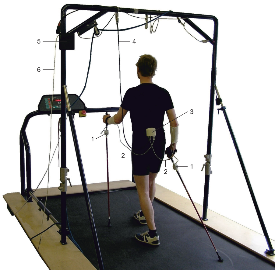
Figure 1 Overview of the system for measuring poling forces. 1 – strain gauge force transducer, 2 – transducer signal cable, 3 – signal conditioning unit, 4 – amplified signal cable, 5 – data acquisition device (AD converter), 6 – USB cable to personal computer. The treadmill was stopped and the safety harness was removed when the photograph was taken.
